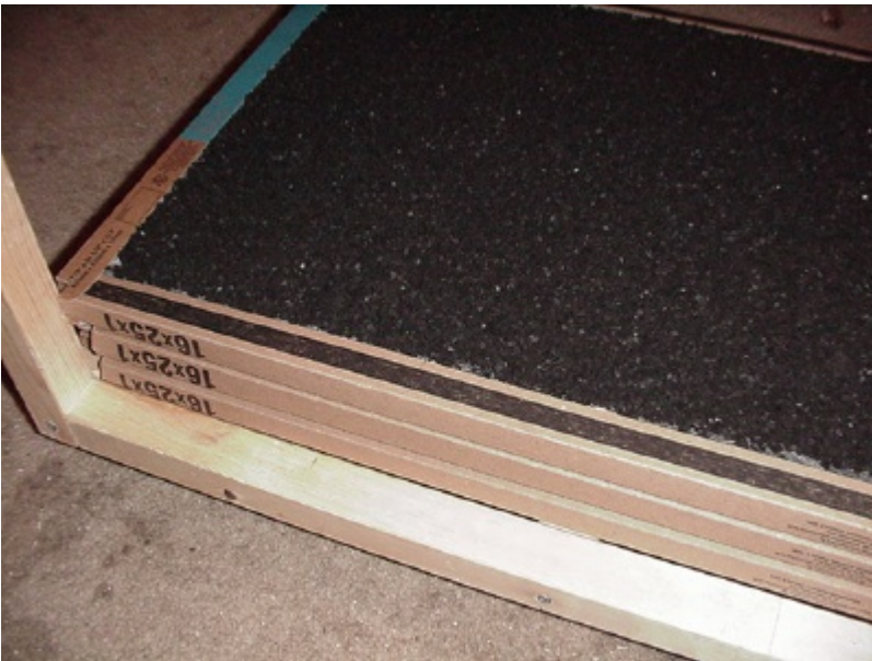
Tape up the carbon/screen layers, and then tape to the base, creating a completely sealed bottom.
